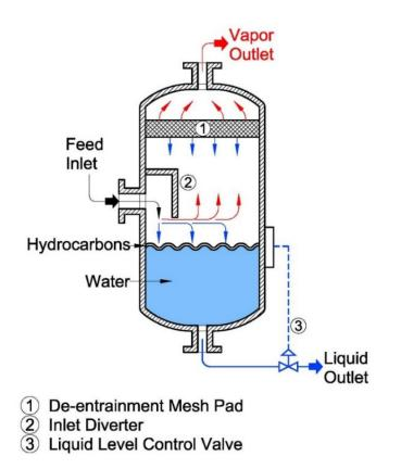
Figure 1. Schematic description of a typical VLL Separator.
