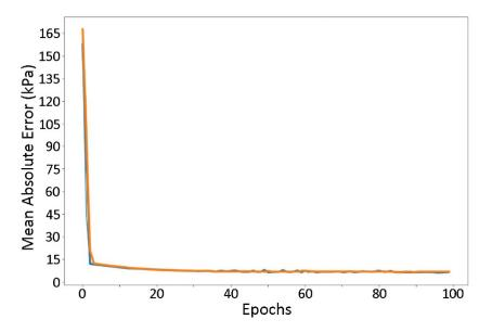
**Figure A2.** Changes of the Pressure Mean Absolute Error with the number of epochs. Notes: Blue curve represent the ANN results following training, and Orange curve describes the ANN results following model validation.
