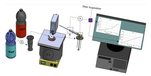
Figure 3. Schematic diagram of CREC-VL-Cell Dynamic Experimental Method. Notes: (1,2): stirring hot plate and aluminum vessel, (3) water and octane, (4) CREC-VL Cell, (5) impeller and thermocouples [8].
