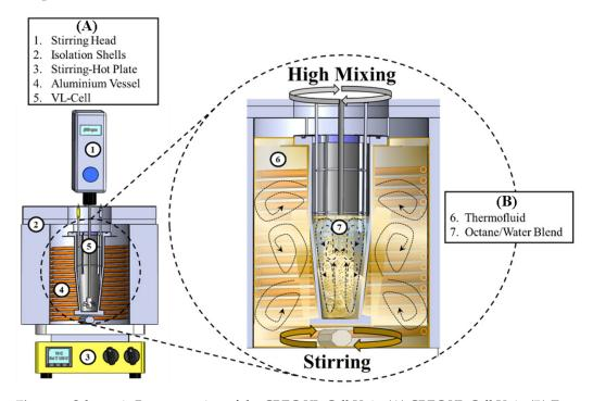
**Figure 2.** Schematic Representation of the CREC-VL-Cell Unit: (**A**) CREC VL Cell Unit, (**B**) Zoom of mixing in the CREC VL Cell. Notes: (1) Stirring Head, (2) Isolation Shells, (3) Stirring Hot Plate, (4) Aluminum Vessel, (5) VL-Cell, (6) Thermofield, and (7) Octane/water Blend [6].
