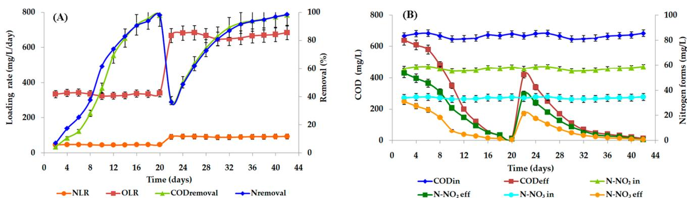
**Figure 4.** The experimental data and calculated parameters of bioconversion in the UASB reactor of media obtained after alkaline hydrolysis of NCS: Reactor and Calculated parameters (A); Influent and Effluent parameters (B).
