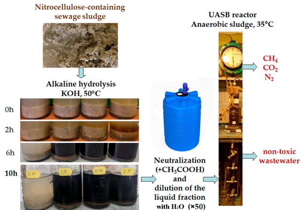
**Figure 1.** Schema of the hybrid chemical-biocatalytic approach for the treatment of NCS from a real chemical industrial complex.
