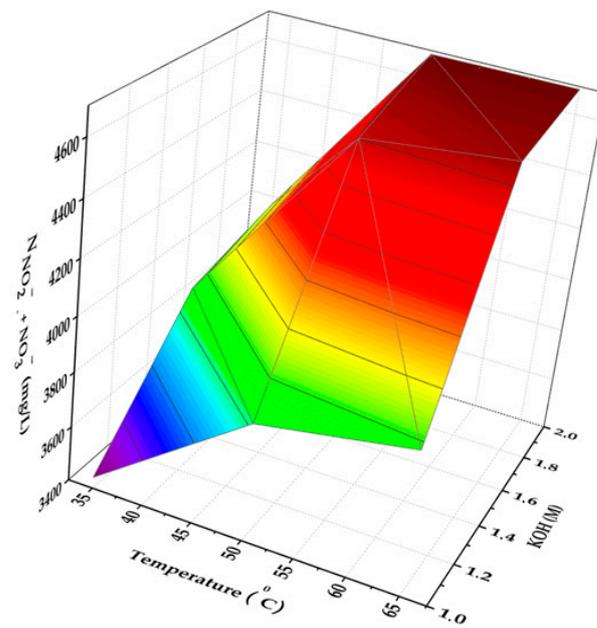
**Figure 2.** Results of accumulation of nitrite and nitrate ions in the liquid fraction under various conditions of NCS alkaline hydrolysis.
