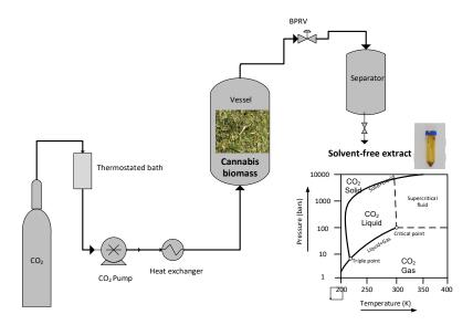
Figure 1. Supercritical carbon dioxide extraction unit.
