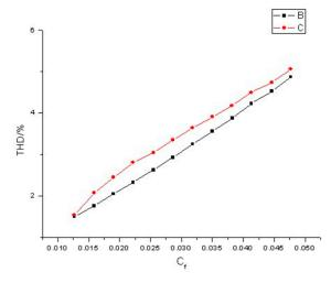
**Figure 6.** Relationship between  $C_f$  and THD (B—proposed improved method; C—conventional AFD method).
