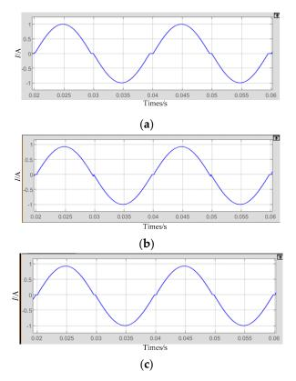
**Figure 8.** Simulation current waveform of conventional AFD and the proposed method. (**a**) is current waveform of conventional AFD, (**b**) is current waveform of the proposed method and (**c**) is current waveform of the proposed improved methods when  $\alpha = 0.08$ .
