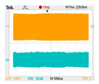
Figure 25. Voltage and current during normal operation of the power grid.
