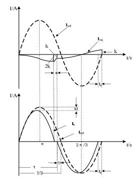
Figure 4. Improved current waveform.
