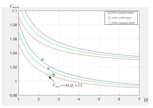
**Figure 5.** NDZ for different  $C_{norm}$ . (The non-detection zone with k = 0.09, k = 0.15 are a and c, respectively; b is the distribution of the non-detection zone with  $C_f = 0.046$  of the conventional AFD method).
