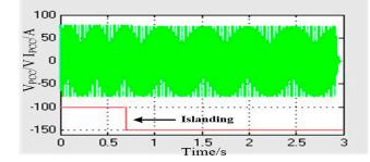
Figure 9. Result of conventional AFD method.
