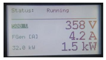
Figure 24. State parameters of the inverter after stabilization.
