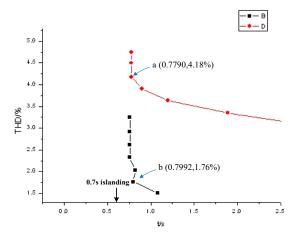
**Figure 7.** Relationship curve between THD and detection time (B—proposed method; D—conventional AFD method).
