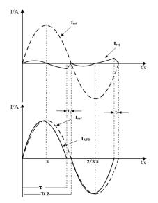
Figure 2. Current waveform of AFD.
