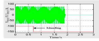
Figure 13. Result of conventional AFD.
