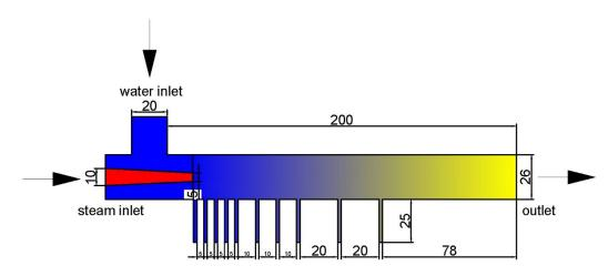
Figure 2. Dimensions of the test section.
