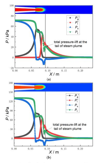
**Figure 8.** The profiles of total pressure, static pressure and dynamic pressure along axial direction.  $G_e = 255 \text{ kg/(m^2 \cdot s)}, T_w = 6.85 \text{ °C}, \text{ and } Re = 19,800;$  (b)  $G_e = 356 \text{ kg/(m^2 \cdot s)}, T_w = 6.85 \text{ °C}, \text{ and } Re = 26,020.$
