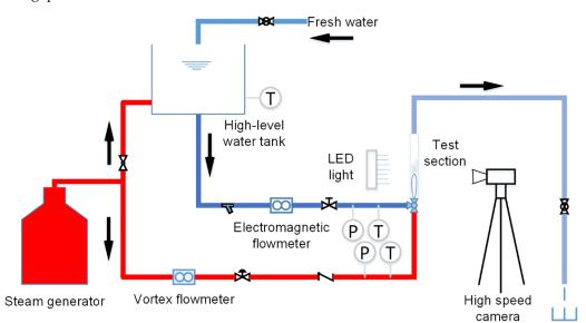
Figure 1. Schematic diagram of experimental system.
