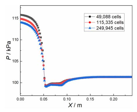
**Figure 4.** Mesh independency check, when  $m_{\beta} = 0.001$  kg/s,  $T_{\beta} = 376$  K,  $m_{\alpha} = 0.05$  kg/s, and  $T_{\alpha} = 300$  K.
