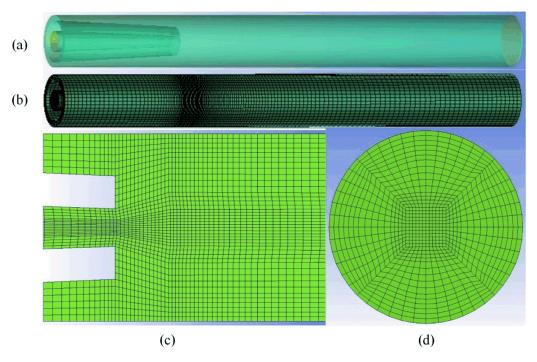
Figure 3. Simulation domain and mesh. (a) Schematic model of simulation domain. (b) Overall geometry showing external surface mesh. (c) Local mesh detail in axial section. (d) Local mesh detail in radial section.
