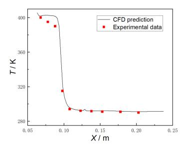
**Figure 6.** Comparison of axial temperature profiles between simulation and experiment [16],  $G_e = 509 \text{ kg}/(\text{m}^2 \cdot \text{s})$ ,  $T_w = 5.9 \text{ °C}$ , and Re = 28,014.
