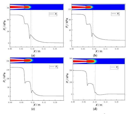
**Figure 7.** The profile of total pressure along axial location. (a)  $G_e = 255 \text{ kg/(m}^2 \cdot \text{s})$ ,  $T_w = 6.85 \,^{\circ}\text{C}$ , and Re = 19,800; (b)  $G_e = 306 \text{ kg/(m}^2 \cdot \text{s})$ ,  $T_w = 6.85 \,^{\circ}\text{C}$ , and Re = 23,850; (c)  $G_e = 407 \text{ kg/(m}^2 \cdot \text{s})$ ,  $T_w = 26.85 \,^{\circ}\text{C}$ , and Re = 28,050; (d)  $G_e = 458 \text{ kg/(m}^2 \cdot \text{s})$ ,  $T_w = 42 \,^{\circ}\text{C}$ , and Re = 28,050.
