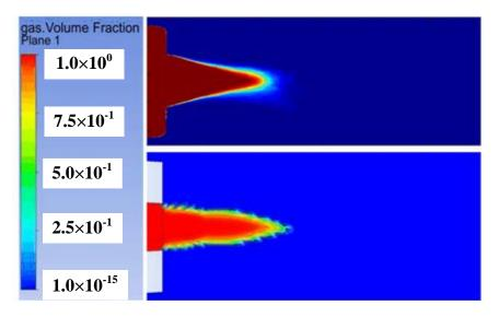
**Figure 5.** Comparison of gas volume fraction between experiment [22] and simulation when  $G_e = 509 \text{ kg/(m}^2 \cdot \text{s})$ ,  $T_w = 5.9 \text{ }^\circ\text{C}$ , and Re = 28,014.
