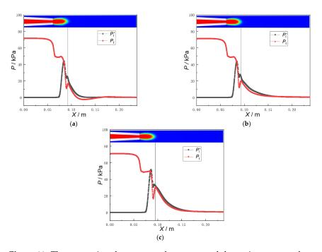
**Figure 11.** The comparison between total pressure and dynamic pressure of water along the axis under different Reynolds numbers of waterflow. (a) Re = 9500; (b) Re = 19,800; (c) Re = 25,000.
