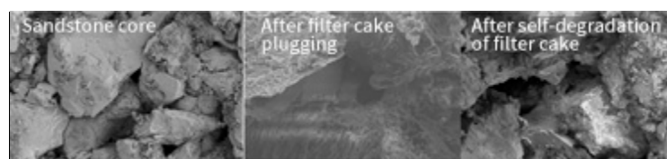
Figure 8. The microstructure of natural sandstone before plugging and after plugging removal.
