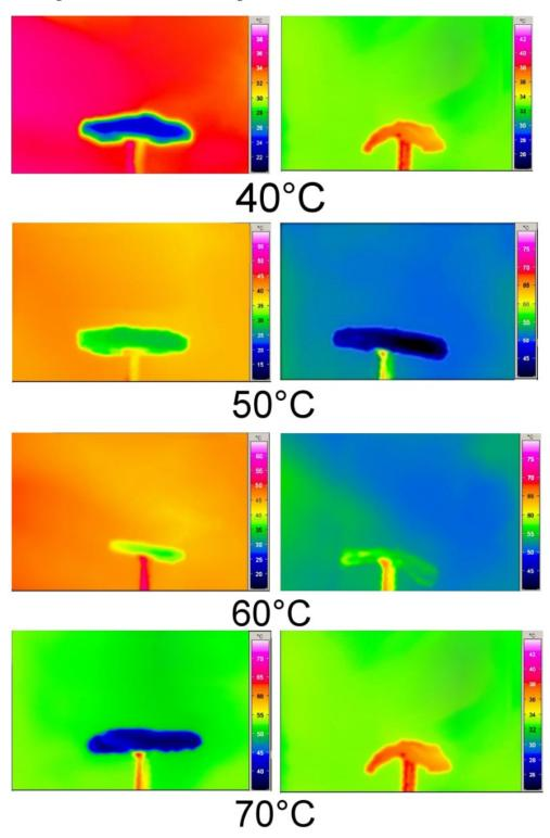
**Figure 6.** Temperature profile and shrinkage behavior for banana slices during the beginning and the end of drying process at different air temperatures with constant air velocity of 0.75 m/s.
