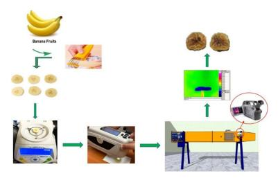
Figure 1. Flowchart describes the applied methodology of monitoring for drying kinetics.
