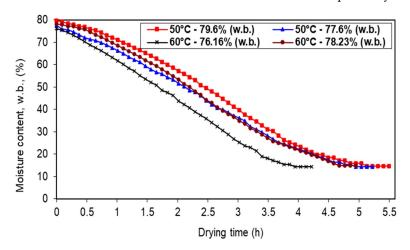
**Figure 10.** Effect of the initial moisture content w.b. on the drying banana slices 2 mm under the same conditions (drying air temperature 50 °C and 60 °C, air velocity 0.75 m/s, and air relative humidity 5–7%).
