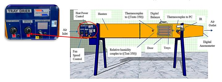
Figure 2. Schematic view of a convection scale single-layer dryer.
