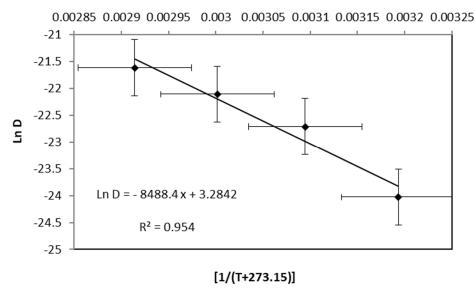
**Figure 11.** ln ( $D_{eff}$ ) for banana slices versus  $1/(T_C + 273.15)$ .
