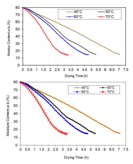
**Figure 5.** Effect of the drying air temperatures under the same conditions (initial moisture content, w.b. 80%, air velocity 0.75 m/s, air relative humidity 5%, and 2 mm thickness of banana slices).
