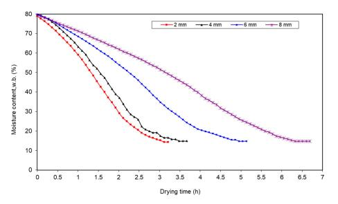
**Figure 9.** Effect of the banana slices thickness under the same conditions (initial moisture content, w.b. 79%, air temperature 70  $^{\circ}$ C, air velocity 0.75 m/s, and air relative humidity 5–7%).
