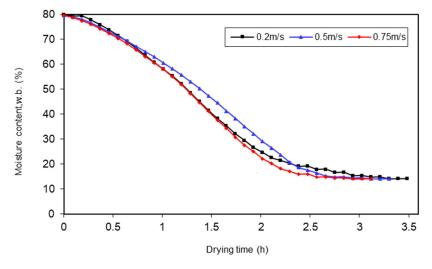
**Figure 8.** Effect of the air velocity under the same conditions (initial moisture content, w.b. 80%, air temperature 70  $^{\circ}$ C, air relative humidity 5–7%, and 2 mm thick banana slices).
