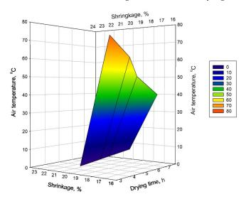
**Figure 7.** Effect of the drying air temperatures on the drying time (h) and the shrinkage % for 2 mm thick banana slices.
