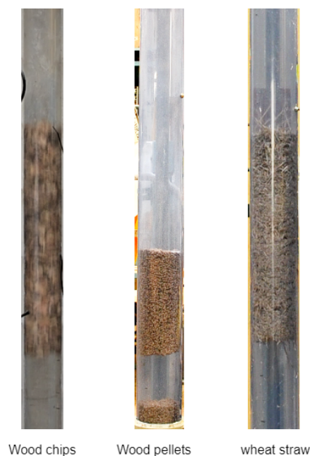
Figure 4. Plug formation in wood chips, wood pellets, and wheat straw.
