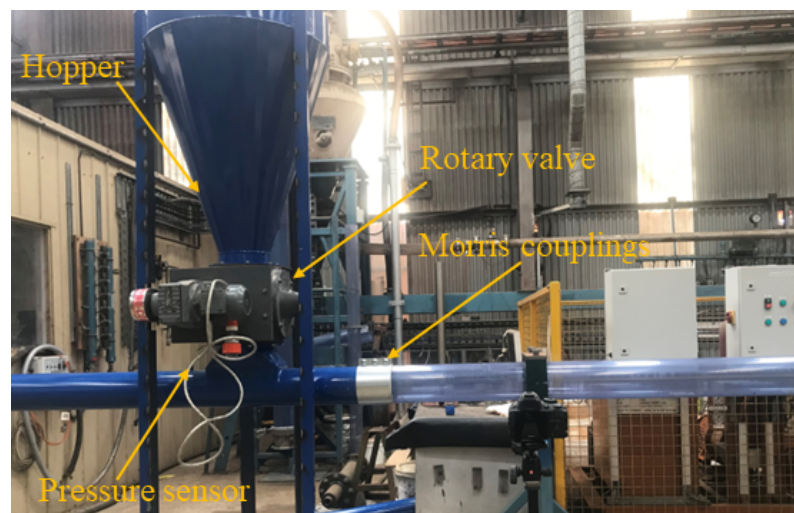
Figure 3. Assembly of the hopper and rotary valve.
