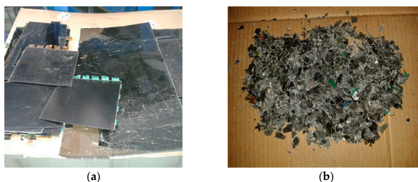
Figure 1. (a) Obtained waste LCD screens; (b) shredded waste LCD screens.
