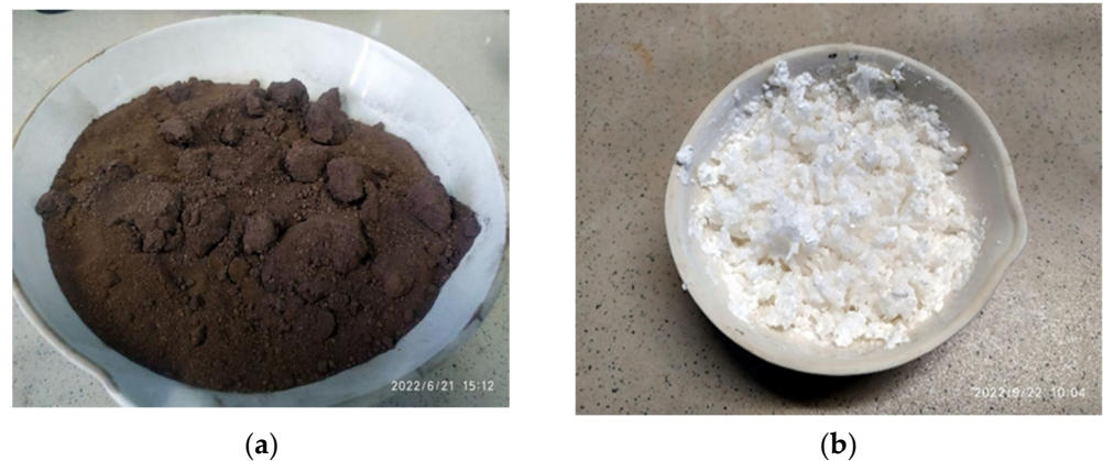
Figure 5. Photos of products: (a) chrome cakes and (b) ammoshenite from chemical processing of DOMPP tailings.
