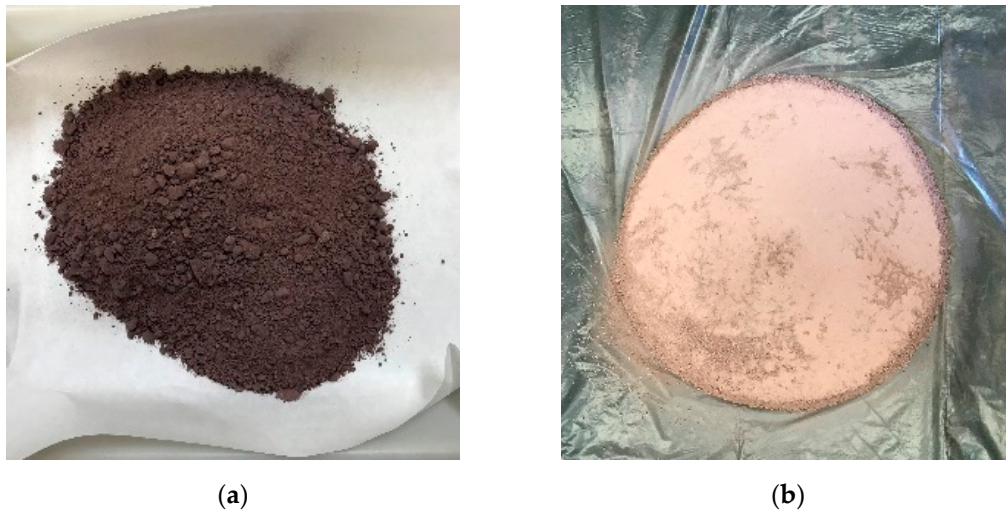
Figure 3. Sample preparation. (a) Sample “as found” [own elaboration]; (b) Sample sieved and homogenized [own elaboration].
