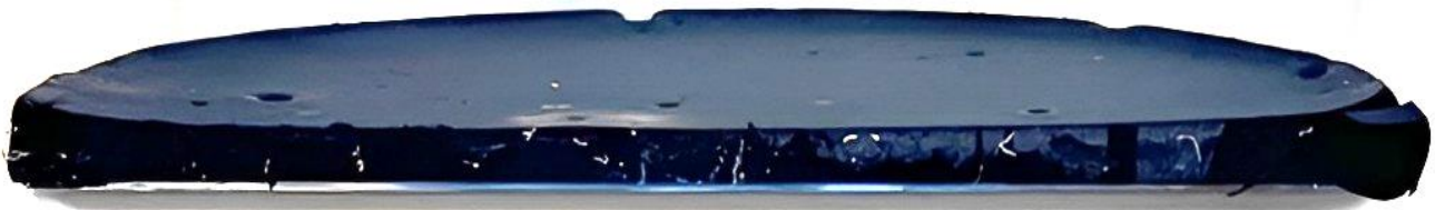
Figure 4. Tilted view of cleaved full 4" size VACNT growth wafer grown at the optimum process condition summarized as Process C.
