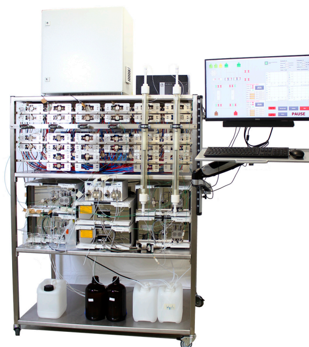
Figure 8. Multi-purpose continuous chromatography prototype.
