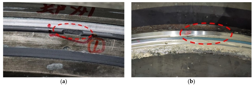
Figure 3. Shear fracture and tear off of sealing ring. (a) Shear fracture of the seal. (b) Tear off of the sealing ring.
