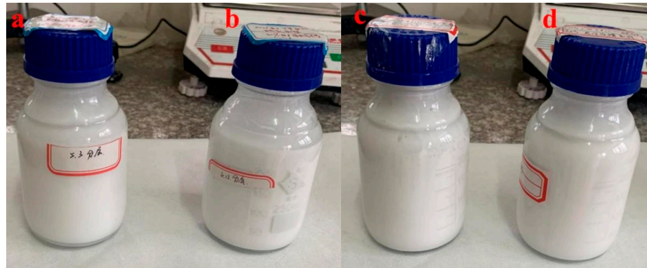
Figure 2. Emulsified suspensions of (a) 30% TBP with \text{Ca}(\text{OH})_2 , (b) 60% TBP with \text{Ca}(\text{OH})_2 , (c) 30% TBP with \text{Mg}(\text{OH})_2 , and (d) 60% TBP with \text{Mg}(\text{OH})_2 .
