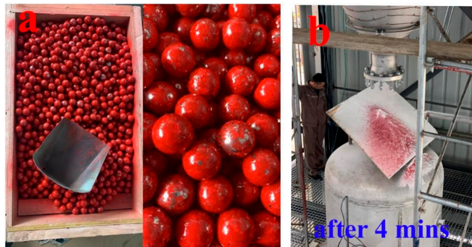
Figure 7. (a) Red-pigment-painted grinding balls and (b) ash hopper (after 4 min operation).
