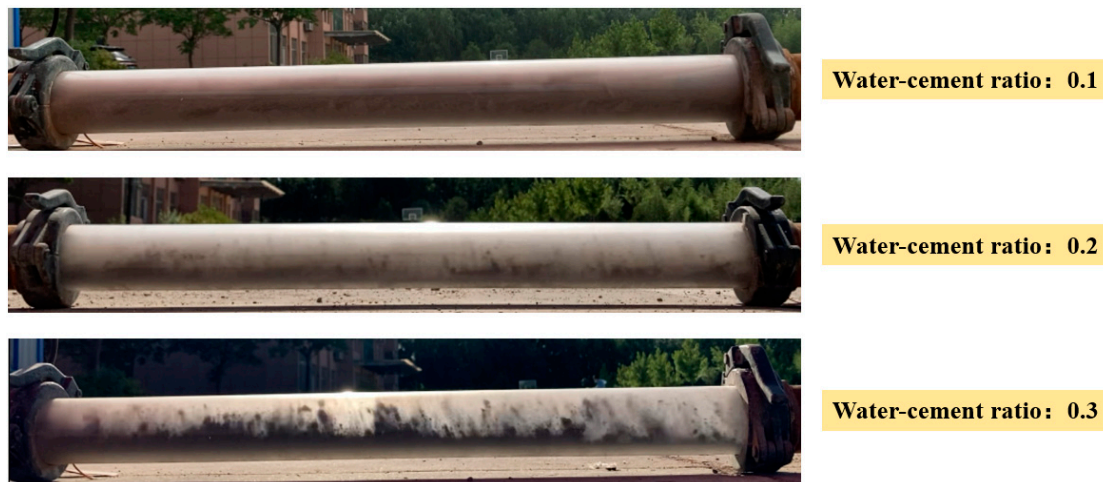
Figure 11. The flow characteristics of stiff shotcrete particles under different water-cement ratios.
