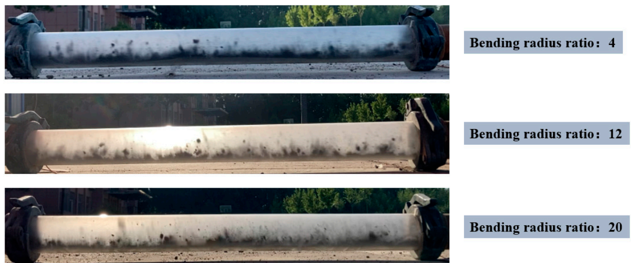
Figure 10. The flow characteristics of stiff shotcrete particles under different bending-diameter ratios.
