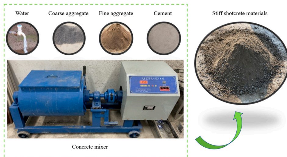
Figure 1. The production process of stiff shotcrete materials.
