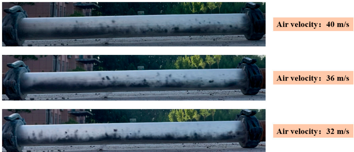
Figure 9. The flow characteristics of stiff shotcrete particles at different air velocities.
