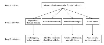
Figure 1. The Green evaluation system of flotation collector.
