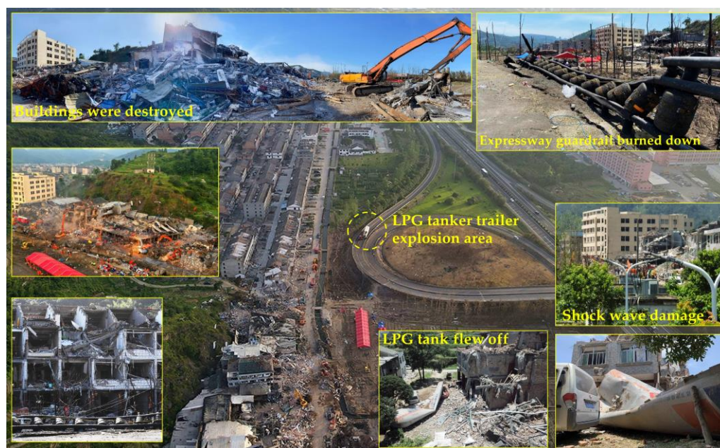
Figure 2. Catastrophic consequences caused by LPG tank trailer explosion in expressway.
