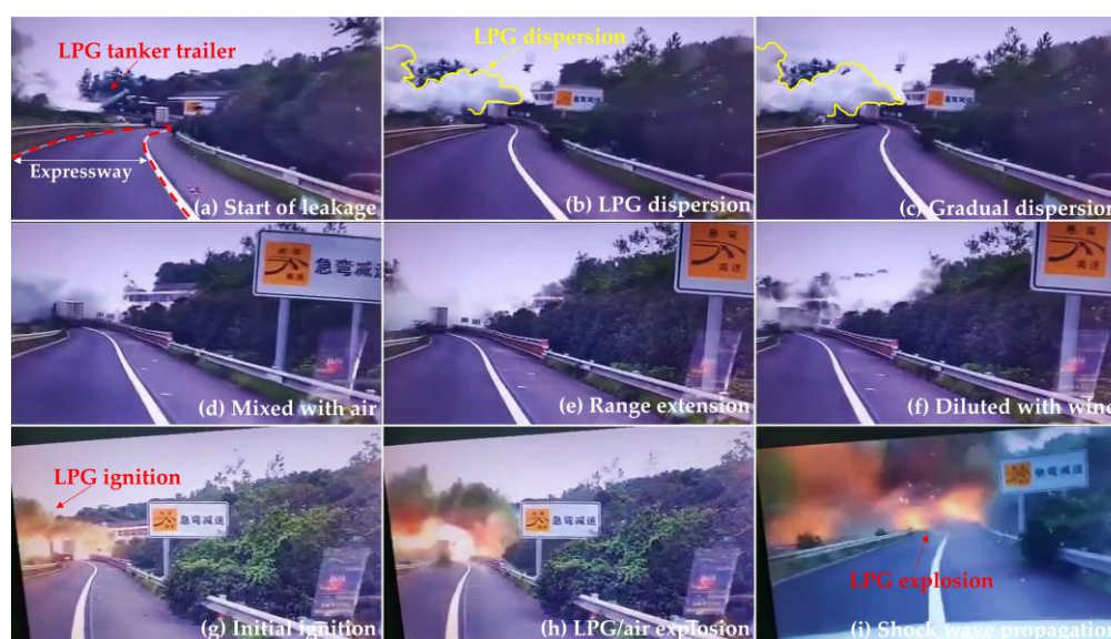
Figure 1. Accidental chain of the LPG tank trailer failures and explodes in expressway transport.
