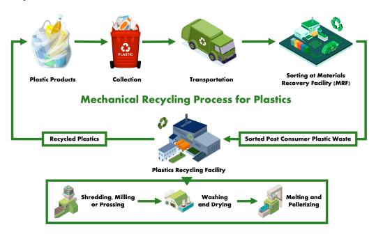
Figure 3. Modern mechanical recycling process for plastic waste.
