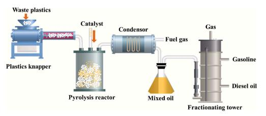
**Figure 4.** Flowchart of plastic waste pyrolysis process. Reproduced with permission from Maqsood, et al. [112]: "Pyrolysis of plastic species: A review of resources and products", published by Elsevier B.V, 2021.
