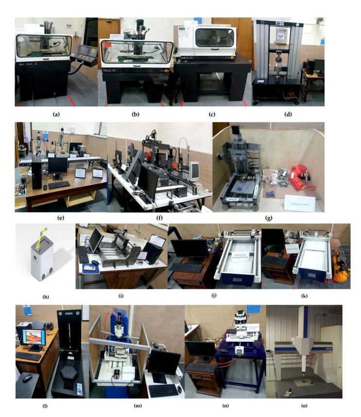
**Figure 9.** (a) CNC milling 1; (b) CNC milling 2; (c) CNC turning; (d) universal tensile testing machine; (e) FMC indigenous; (f) FMC retrofitted; (g) pneumatic jet printer; (h) automated guided vehicle (Cobot); (i) precision router; (j) selective laser sintering 3D printer; (k) binder jet; (l) 3D laser scanner; (m) five axis CNC milling machine; (n) electro-hydrodynamic jet printer; and (o) coordinate measuring machine.
