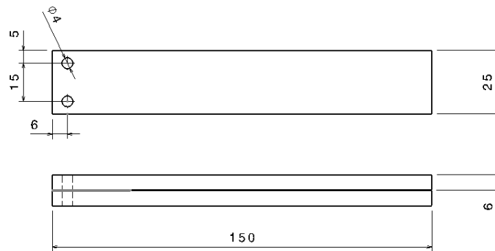
Figure 3. Composite DCB geometry.
