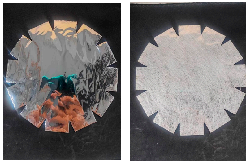
Figure 1. The reflector and spacer of the MLI.
