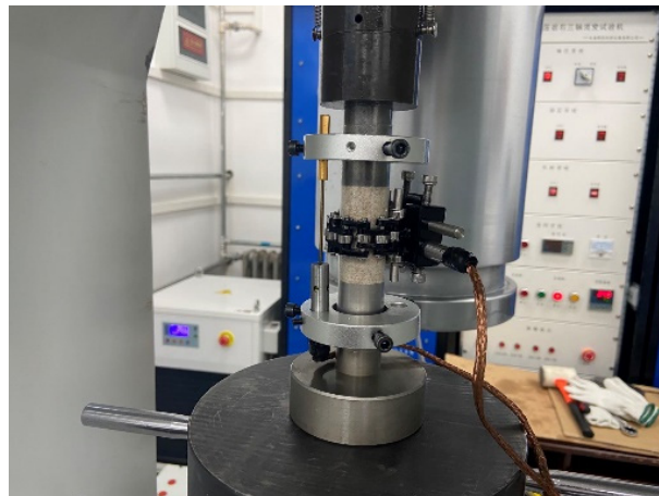
Figure 1. Uniaxial compression test by TAR-1500 Rock mechanics test system.
