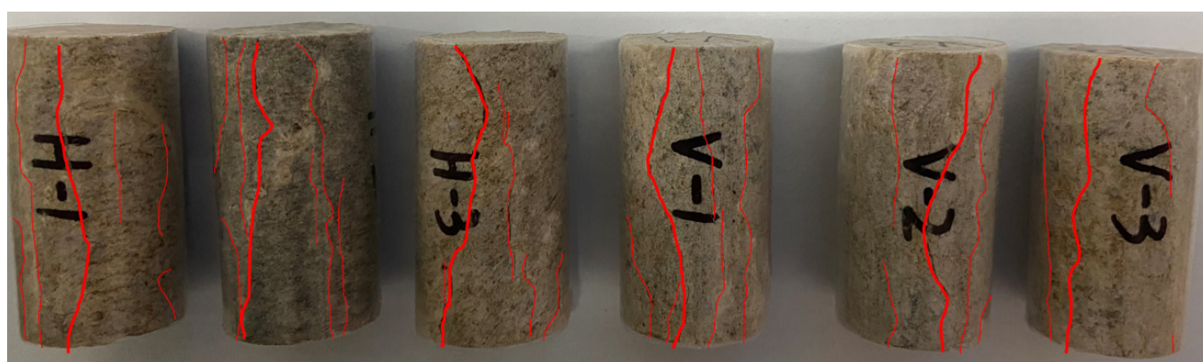
Figure 6. The gneiss specimens after compression. (The red lines are cracks).
