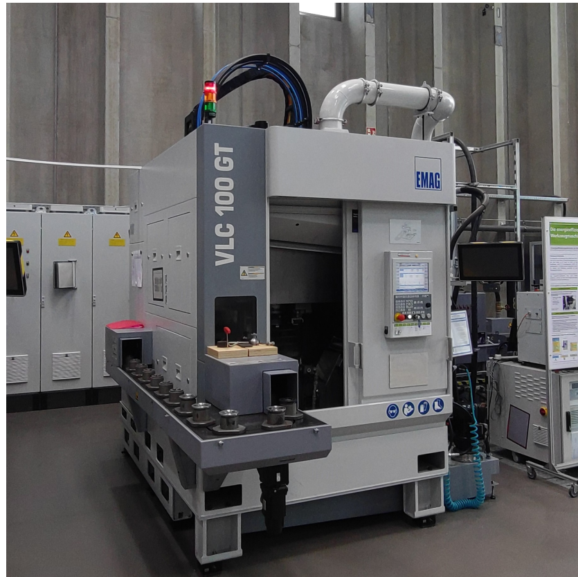
Figure 3. Picture of the CNC grinding machine of the use case for the energy-flexible operation.
