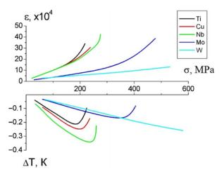
**Figure 1.** Dependence of deformations  $\varepsilon$  and temperature changes  $\Delta T$  of samples on mechanical stresses  $\sigma$  [31] (the temperature is measured by additional thermocouple touched to the sample).
