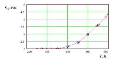
**Figure 3.** Temperature dependence of the sensitivity of the thermocouple  $Fe_{40}Ni_{40}P_{14}B_6/Fe_{80}Cu_3B_{17}$  (blue points for experimental data, red points for estimated data).
