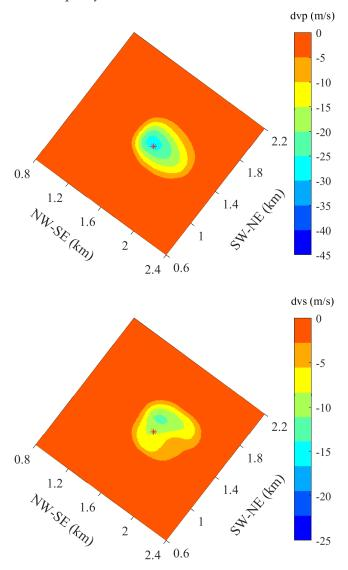
**Figure 10.** Inverted time-lapse velocity changes between baseline and Monitor 1 VSP surveys at the center depth of Morrow B. The red asterisk labels the VSP/injection-well position.
