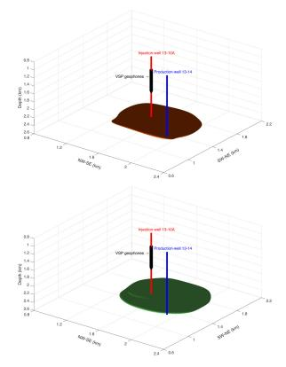
**Figure 16.** The volumetric contours of inverted time-lapse velocity changes between baseline and Monitor 2 VSP surveys, where brown and green colors indicate  $V_p$  and  $V_s$  changes, respectively.
