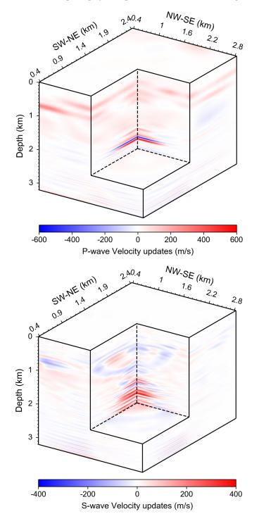
**Figure 8.** Velocity updates obtained using 3D elastic-waveform inversion of 3C VSP upgoing waves of the baseline VSP data (i.e., differences by subtracting models in Figure 6 from those in Figure 7), with both low-wavenumber tomographic and high-resolution detailed updates.
