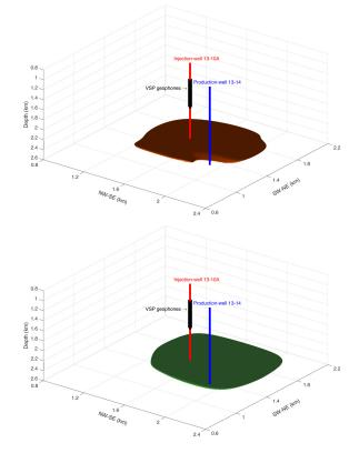
**Figure 17.** The volumetric contours of inverted time-lapse velocity changes between baseline and Monitor 3 VSP surveys, where brown and green colors indicate  $V_p$  and  $V_s$  changes, respectively.
