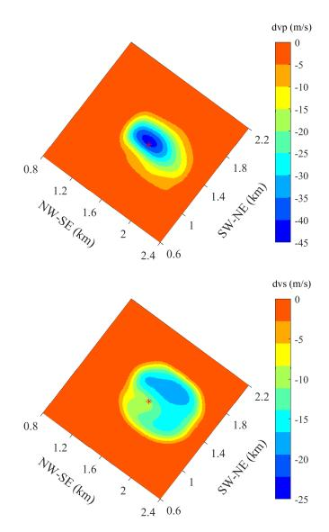
**Figure 11.** Inverted time-lapse velocity changes between baseline and Monitor 2 VSP surveys at the center depth of Morrow B. The red asterisk labels the VSP/injection-well position.
