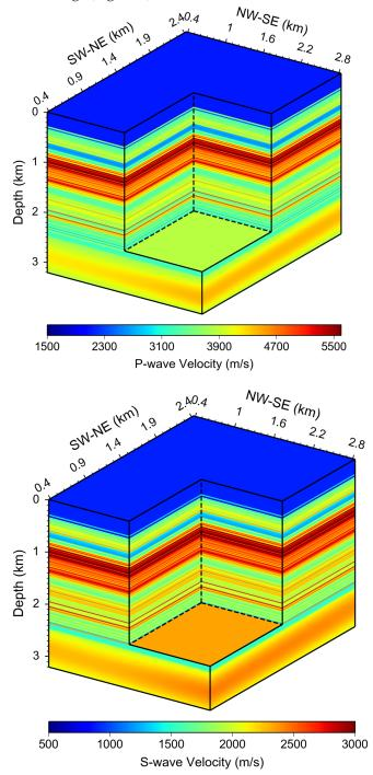
**Figure 5.** Updated baseline  $V_p$  model by incorporating the deep region of the velocity model derived from the 3D surface seismic data and  $V_s$  model with the deep region updated according to the  $V_p/V_s$  ratio at the lower boundary of the sonic logs.
