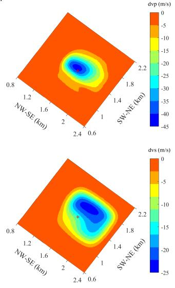
**Figure 12.** Inverted time-lapse velocity changes between baseline and Monitor 3 VSP surveys at the center depth of Morrow B. The red asterisk labels the VSP/injection-well position.
