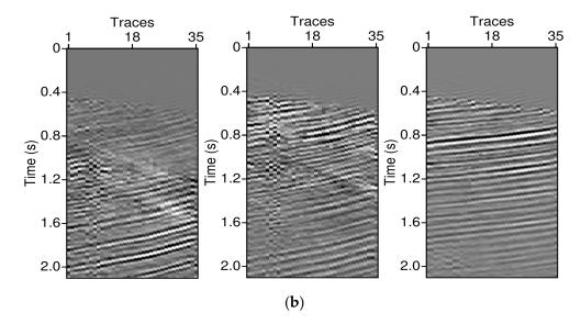
**Figure 2.** Left, middle, and right panels show X (East), Y (North) and Z (Vertical) components, respectively, of (**a**) full wavefield data and (**b**) the separated upgoing data of the baseline 3D-3C VSP survey.
