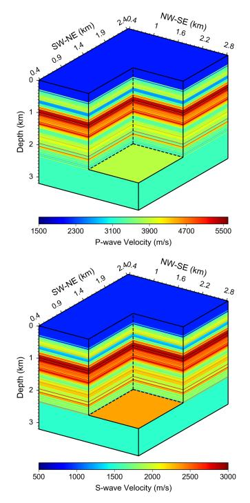
**Figure 4.** Initial baseline P-wave  $(V_p)$  and S-wave  $(V_s)$  velocity models obtained by upscaling the sonic log.
