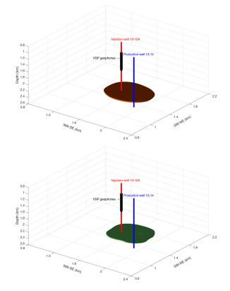
**Figure 15.** The volumetric contours of inverted time-lapse velocity changes between baseline and Monitor 1 VSP surveys, where brown and green colors indicate  $V_p$  and  $V_s$  changes, respectively.
