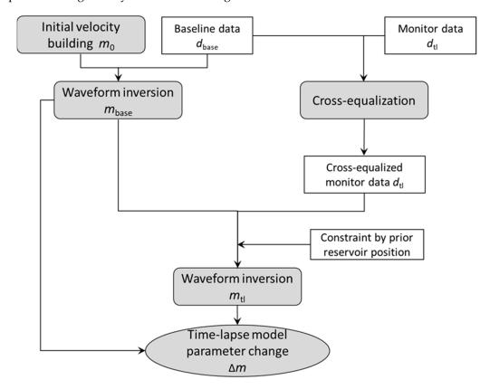
Figure 3. Workflow of time-lapse seismic processing and inversion for time-lapse velocity changes.
