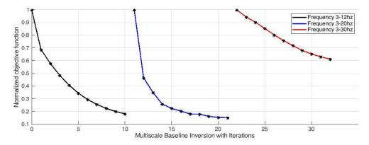
**Figure 9.** Convergence curves of 3D multi-scale elastic-waveform inversion of the baseline VSP data at three frequency scales.
