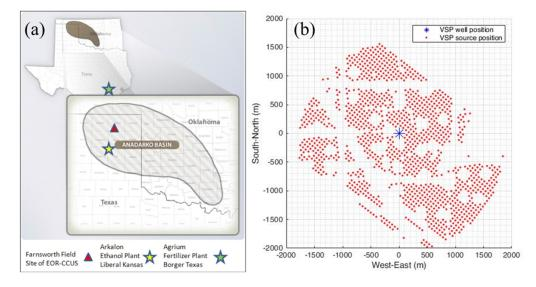
**Figure 1.** (**a**) Location of the Farnsworth CO<sub>2</sub>-EOR field as indicated by the red up-pointing triangle, and (**b**) VSP acquisition geometry for the baseline 3D-3C VSP survey.
