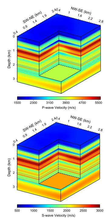
**Figure 6.** Improving the shallow regions of the baseline  $V_p$  model using first-arrival tomography of the downgoing waves of the baseline VSP data, together with  $V_s$  model with estimated updates for the shallow region according to the  $V_p/V_s$  ratios at the upper boundary of the sonic logs.
