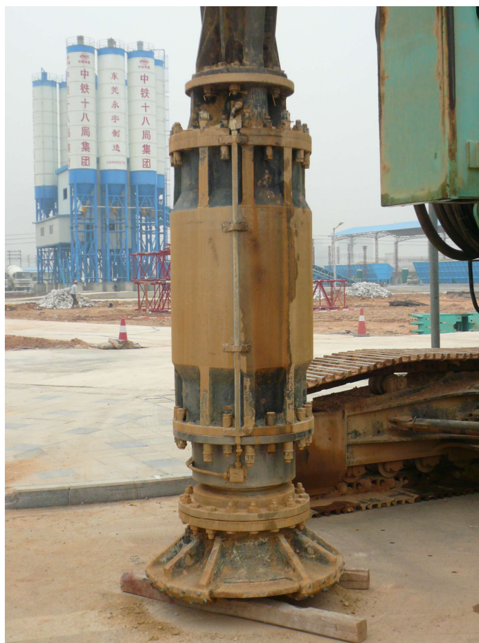
Figure 11. Photographic image of large-diameter DTH hammer and RC drill bit.
