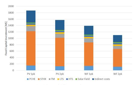
Figure 9. Investment breakdown of different configurations.
