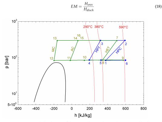
**Figure 7.** Pressure–enthalpy diagram of the proposed Carnot battery (heat pump in blue lines and heat engine in green lines).
