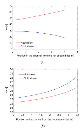
Figure 5. Nusselt number: (a) LTR (146 MW) in the heat engine; (b) REC (266 MW) in the heat pump.
