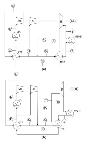
Figure 2. Power cycles (heat engines) recompression layouts: (a) Conventional; (b) Modified.
