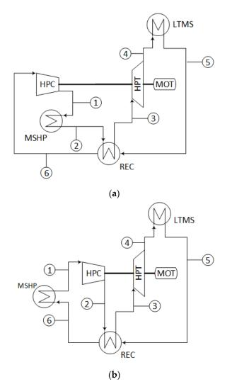
Figure 3. Reverse Brayton cycles (heat pumps) layouts: (a) conventional; (b) modified.
