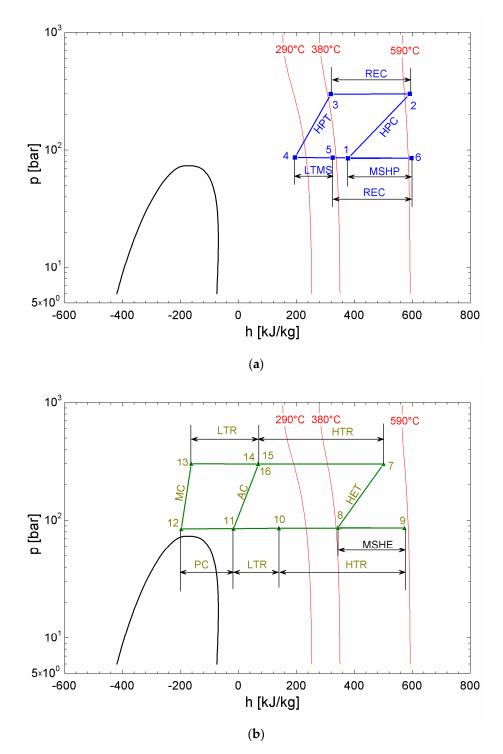
Figure 8. Pressure–enthalpy diagrams: (a) heat pump; (b) heat engine.
