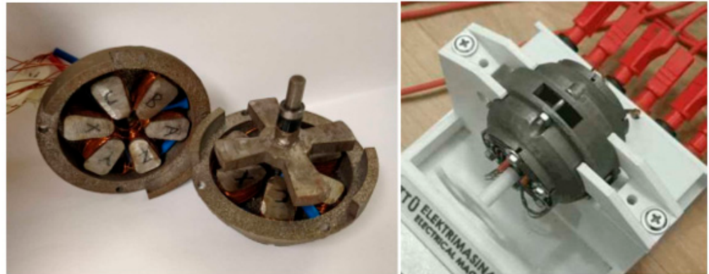
Figure 5. Printed axial machine having stator halved embedded teeth [42].
