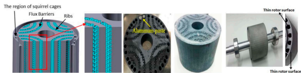
Figure 7. 3D-printed rotor of line start synchronous reluctance machine [46].
