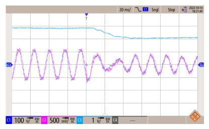
**Figure 12.** Capacitor Bank Capacitance Considered by the Control Algorithm (3) and Filter Capacitor Voltage Response (C1) to Variation in the Capacitor Bank Value with Online Estimation.
