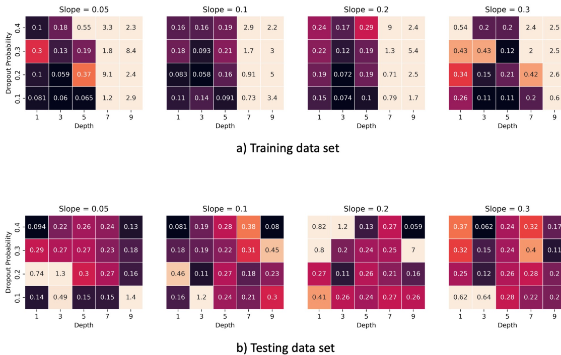
Figure 8. Heat map of the NN showing the corrected cone resistance q_t MSE results obtained for a combination of different depths of network against the slope ( \alpha ) parameter to adjust the leak in the LeakyReLU for the testing data. The results show the tuning of the depth of the NN and slope of the activation function. The annotations in each square represent the averaged MSE for that model. (a) shows the results of the MSE calculated from the different networks on the training data. (b) shows the results of the MSE calculated from the different networks on the testing data.
