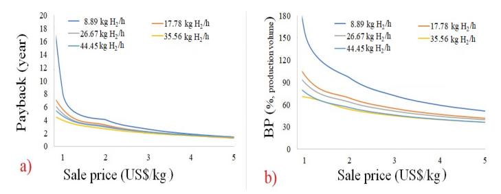
**Figure 4.** Effect of H<sub>2</sub> sale price on the: (**a**) payback and (**b**) break-even point for different production capacities.
