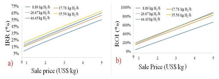
Figure 5. Effect of H<sub>2</sub> sale price on the (a) IRR and (b) ROI for different production scales.
