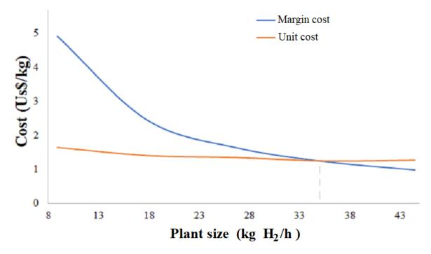
Figure 8. Joint analysis of cost and revenue of hydrogen production project.
