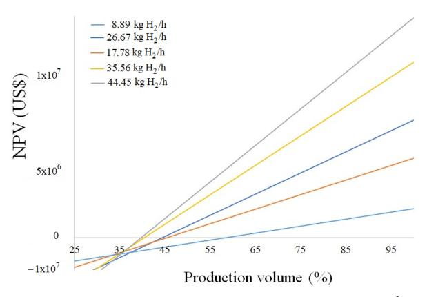
**Figure 7.** NPV variation with production volume at 2 USD/kg  $H_2$  and 5 USD/Nm<sup>3</sup>  $O_2$ .
