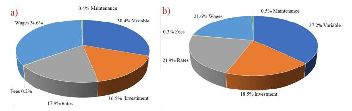
**Figure 3.** Cost composition of hydrogen production plants. (**a**) one electrolysis kit, (**b**) five electrolysis kit.
