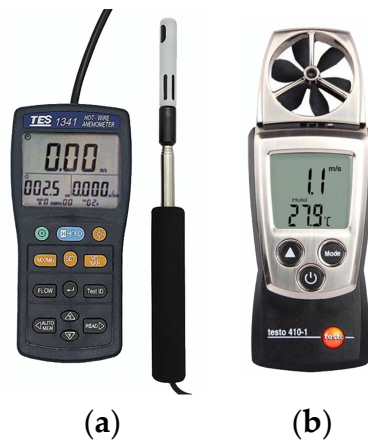
Figure 4. Testing instruments: (a) thermocouple anemometer and (b) impeller anemometer.
