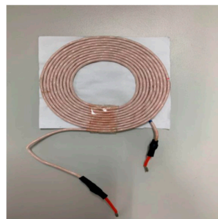
(a) Single-layer proposed transmitter coil
