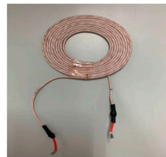
(b) Single-layer proposed receiver coil
