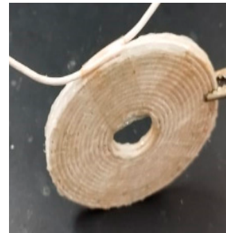
(b) Double-layer receiver coil
