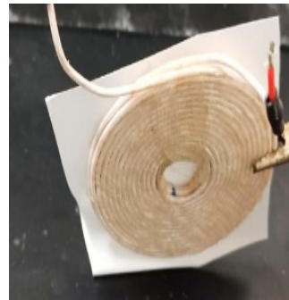
(a) Double-layer transmitter coil
