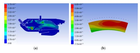
**Figure 13.** Contours of mass fraction of NO in longitudinal section (**a**) and at the outlet (**b**) for combustion chamber with steam injection.
