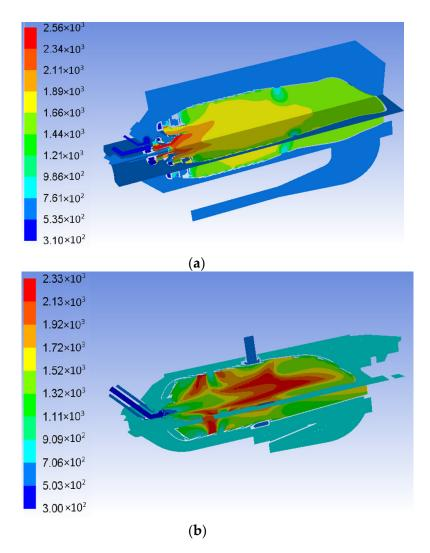
**Figure 9.** Contours of temperature, K, inside the volume of combustion chamber with preliminary component mixing (**a**) and with steam injection (**b**).
