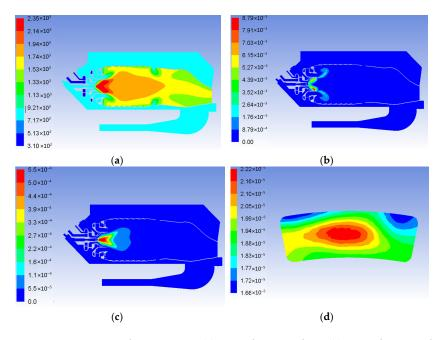
Figure 12. Contours of temperature (a), mass fraction of CO (b), mass fraction of NO (c) in longitudinal section, and mass fraction of NO at the outlet (d) for the premixed combustion chamber at 20%  $H_2$  (by volume).
