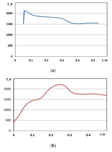
**Figure 10.** Temperature distribution along the flame tube length for the combustion chamber with preliminary component mixing (**a**) and with steam injection (**b**).
