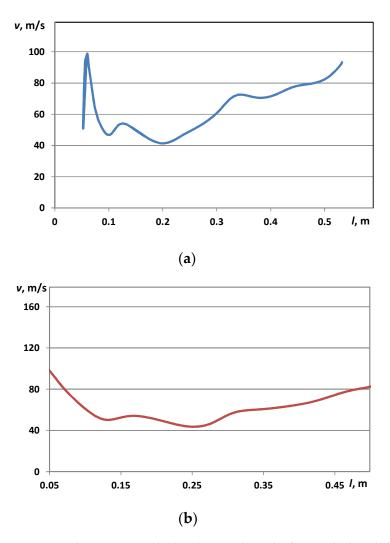
**Figure 8.** Velocity magnitude distribution along the flame tube length for the combustion chamber with preliminary component mixing (**a**) and with steam injection (**b**).
