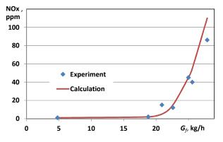
**Figure 4.** Concentrations of NOx at the outlet of the combustion chamber with preliminary mixing of the components.
