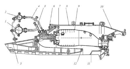
**Figure 2.** Combustion chamber with premixing of components: 1, 2—fuel collectors; 3, 4—fuel supply lines; 5—casing of compressor; 6—burner; 7—spacer; 8—frame; 9—flame tube; 10—turbine casing; 11—diffuser; 12—housing.
