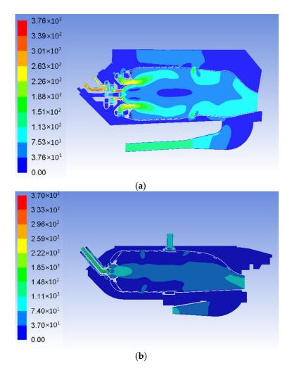
**Figure 7.** Contours of velocity magnitude, m/s, inside the combustion chamber with preliminary component mixing (**a**) and with steam injection (**b**).
