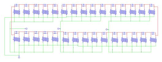
Figure 8. PV array and DC–DC boost converter circuits employed in Psim environment.
