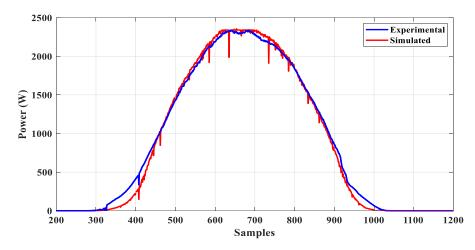
**Figure 15.** Comparison of experimental and simulated powers at MPP under clear conditions using DO-based MPPT.
