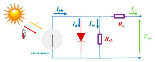
Figure 3. ODM of PV cell.
