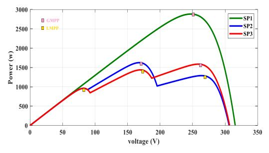
Figure 9. Shading patterns.
