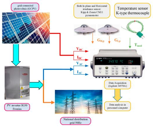
Figure 2. PV study plant and the monitored system.
