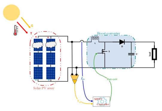
Figure 1. Illustration of PV System with Boost Converter for MPPT.
