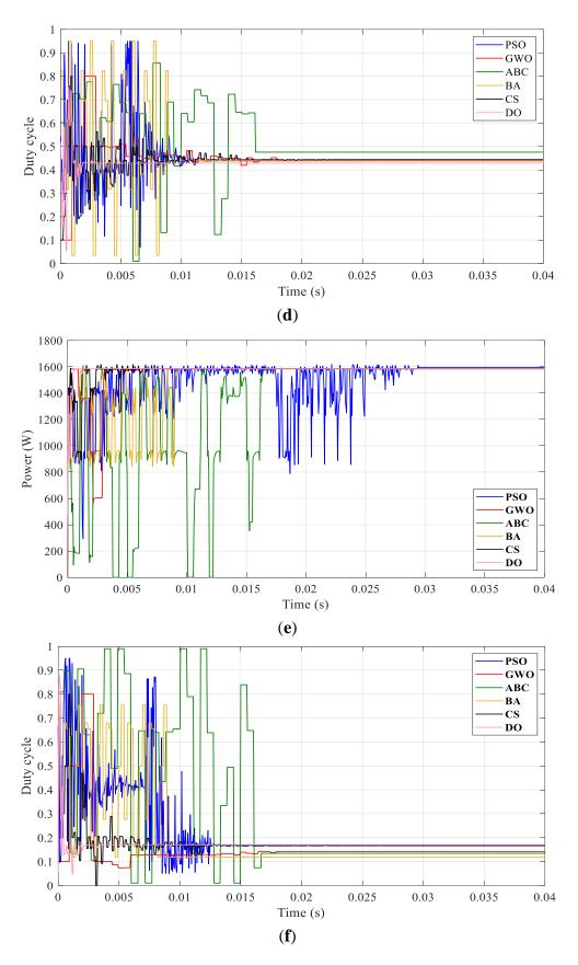
**Figure 10.** Simulated mean power and duty cycle of PSO, GWO, ABC, BA, CS, and DO for PV string ((**a**,**b**) for SP1, (**c**,**d**) for SP2, (**e**,**f**) for SP3).
