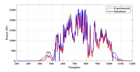
**Figure 16.** Comparison of experimental and simulated powers at MPP under shading conditions using DO-based MPPT.
