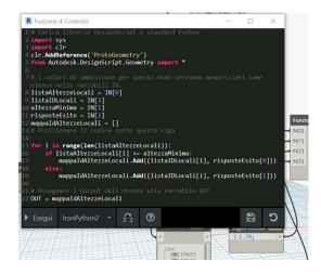
Figure 4. Python script node for control function using the logic described by "IF-ELSE" type rules.
