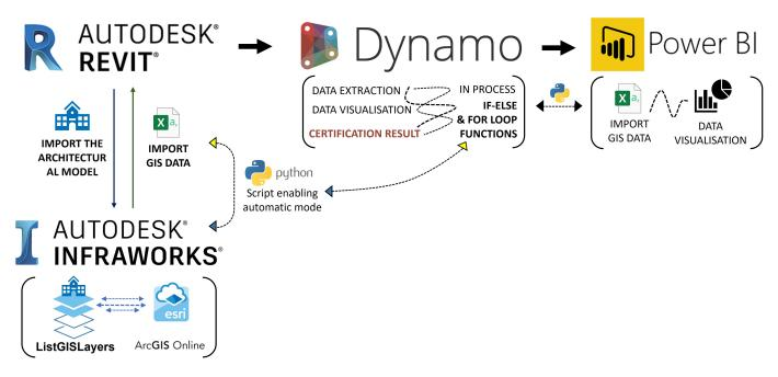
Figure 1. Flowchart of the connection of the BIM model with digital technologies.
