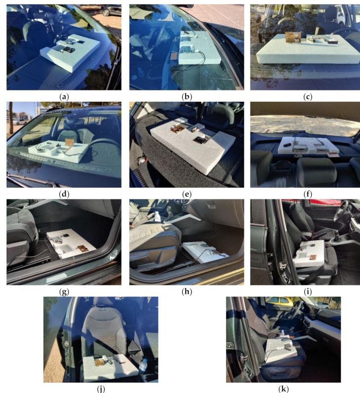
Figure 3. Different positions and orientations in which the devices were arranged inside the vehicle. For (g,h), the seat covered the device. For illustrative purposes, the seat was moved to the back to show both devices. (a) Front Dashboard–Face Up; (b) Front Dashboard–Upside down; (c) Front Dashboard–Face forward; (d) Front Dashboard–Face backward; (e) Rear Dashboard; (f) Rear Dashboard–Upside down; (g) Under the seat; (h) Under the seat–Upside down; (i) Over the seat; (j) Over the seat–Face forward; (k) Over the seat–Upside down.
