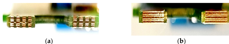
Figure 14. Laminated PCB winding structure. (a) Primary-side laminated PCB winding structure of the transformer and (b) secondary-side laminated PCB winding structure of the transformer.
