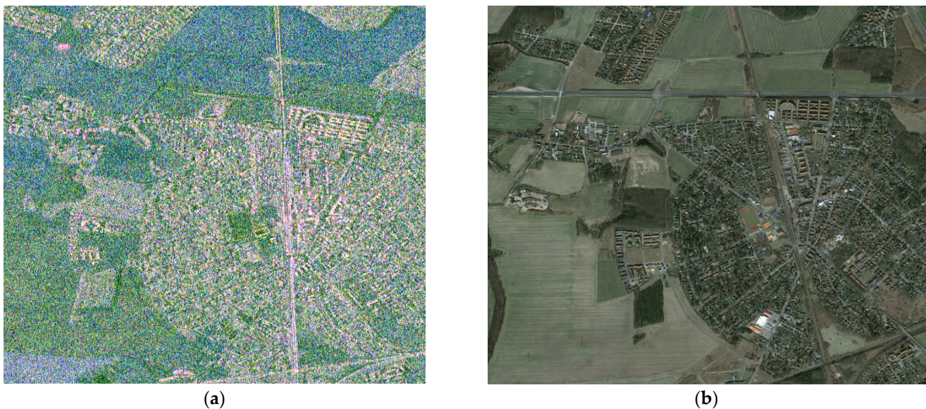
Figure 6. (a): Pauli-coded color composition of polarimetric channels (red: |hh-vv| , green: |hv| , blue: |hh+vv| ). (b): optical image of studied region (source: Google Earth).
