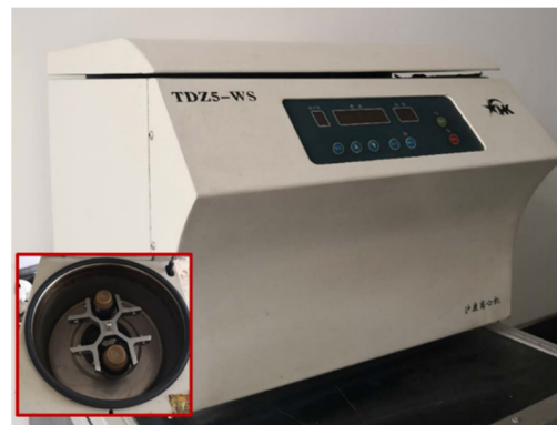
Figure 5. TDZ5-WS centrifuge and its internal structure.
