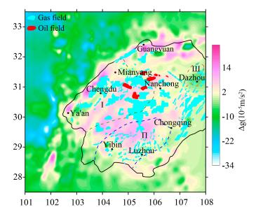
**Figure 7.** Residual anomaly and distribution features of the research area's major oil and gas fields. (I: Leshan–Longnvsi paleo–uplift; II: Luzhou paleo–uplift; III: Kaijiang paleo–uplift).
