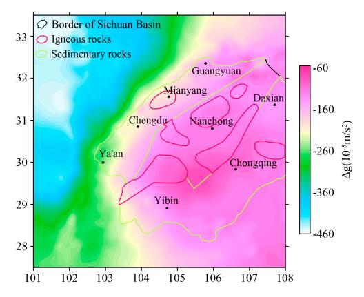
**Figure 2.** Map of the Bouguer gravity anomalies in central and western Sichuan Basin (modified from Zhou [13] and Chen et al. [17]).
