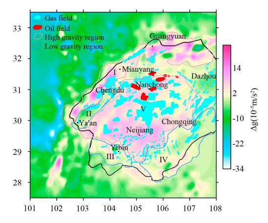
**Figure 3.** Map of the residual gravity anomaly in central and western Sichuan Basin. (I: high gravity value in Longmenshan–Micangshan area; II: the low–value gravity area in Ya 'an; III: the low–value gravity area in Yibin; IV: the low–value gravity area in Huayingshan–Qiyueshan; V: high–value gravity in Neijiang–Nanchong area).
