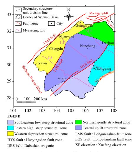
Figure 6. Delineation of tectonic elements of the central and western Sichuan Basin.
