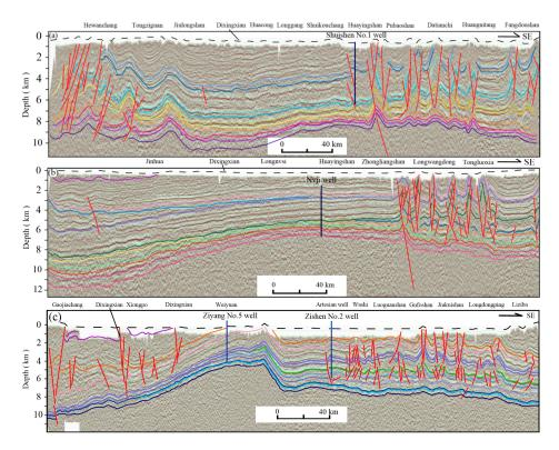
**Figure 5.** The deep seismic reflection profiles of Sichuan Basin (modified from Li [2]). (**a**) L1; (**b**) L2; (**c**) L3.
