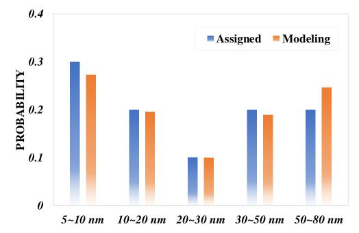
Figure 3. Comparison of the target pore size distribution and that generated by the program.
