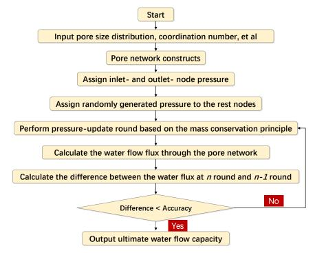
Figure 2. Calculation procedures for pore network modeling on stable water flow.
