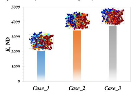
Figure 8. Impact of pore size distribution on apparent permeability.
