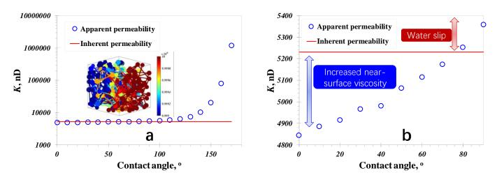
**Figure 4.** Water flow capacity in porous media consisting of nanopores: (**a**) Apparent permeability versus surface contact angle; (**b**) Underlying mechanism governing water flow capacity.
