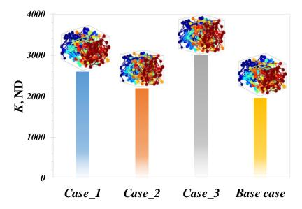
Figure 6. Wettability effect on apparent permeability for water flow at core scale.
