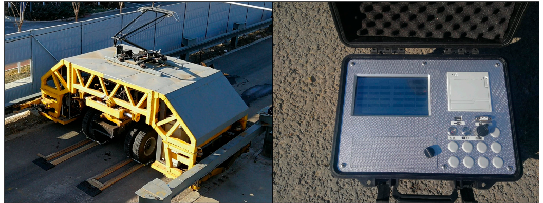
Figure 5. Static axle load measurement of NE-ALT.
