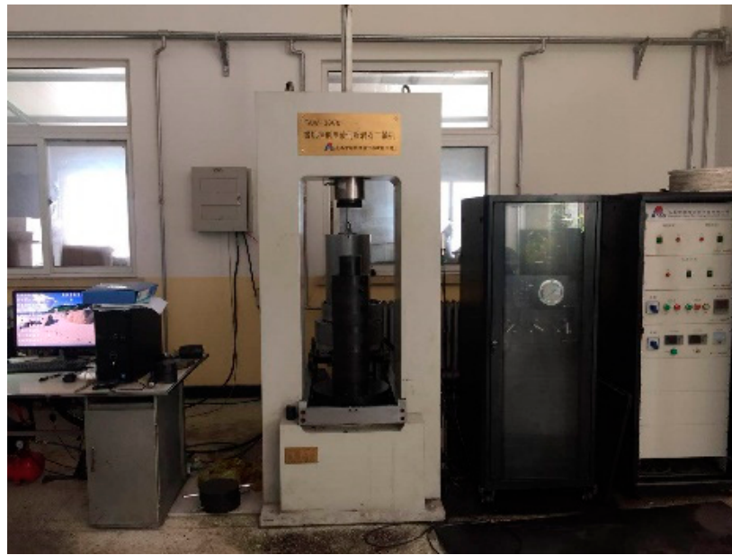
Figure 4. TAW-3000 electro-hydraulic servo rock triaxial testing machine.
