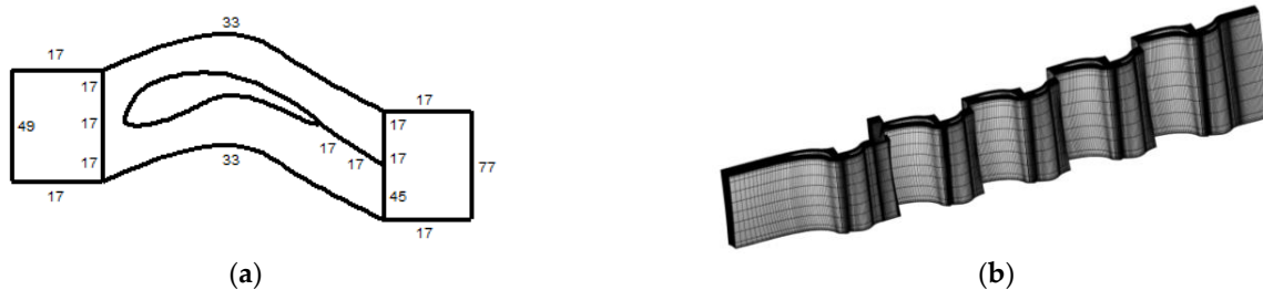
Figure 2. Schematic diagram of model mesh: (a) H-O-H topology; (b) computational grid.
