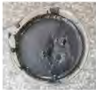
Figure 3. Particle size grading scheme 1: paste with 75% mass fraction.
