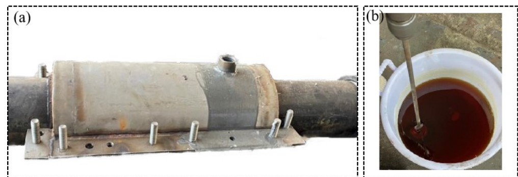
Figure 2. Test materials and setup: (a) offshore oil transfer conduit and exterior sleeve construction; (b) dispensing condition for plugging agents.
