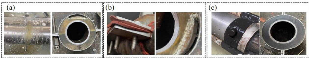
Figure 7. Plugging agent dispensing test: (a) the plugging agent leaking and not being in a fully filled state after curing; (b) the improved sleeve closure and plugging agent micro-crack state; and (c) the plugging agent curing success state.
