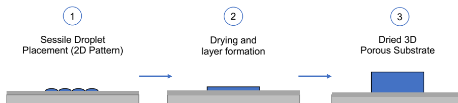
Figure 1. Simplified scheme of porous substrate formation by layer-by-layer build-up from single droplet deposits (repeated execution of steps 1 and 2). The liquid of the droplets is evaporated into a heated gas.
