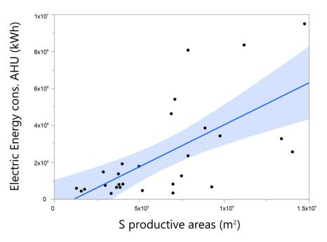
Figure 9. Correlation between electricity AHU consumption and surface of production areas [m<sup>2</sup>].
