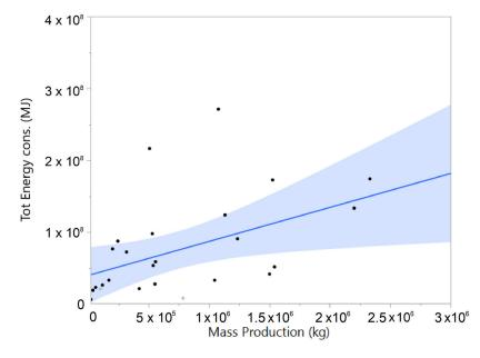
Figure 6. Distribution of the total energy consumption [MJ] vs. mass production [kg].
