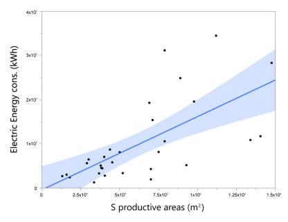
**Figure 7.** Distribution of the electric energy consumption [kWh] vs. surface of production areas [m<sup>2</sup>].
