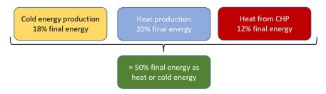
**Figure 5.** Estimation of the mean amount of final energy consumed as heat or cold energy in a pharmaceutical plant: around 50% of the final energy comes as heat or cold energy.
